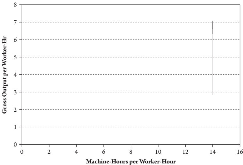
Figure 4.13 Output per Worker-Hour versus Machine-Hours per Worker-Hour, for 8-Hour Shifts Operated up to Engineering Capacity (Two and a Half Shifts)
