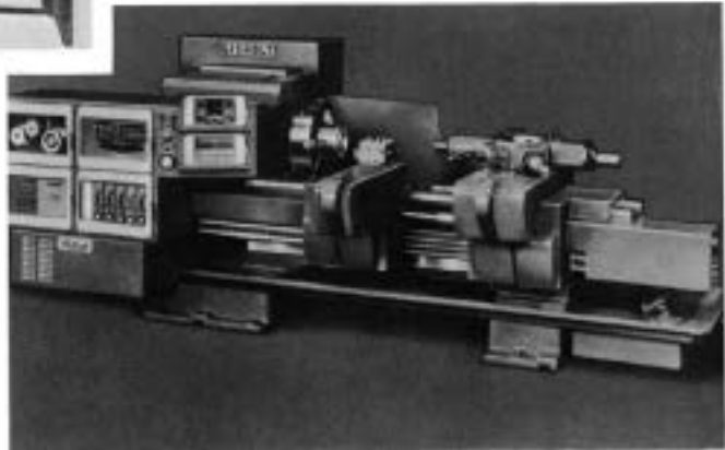
Gisholt Factrol lathe with record-playback control system conceived by Leif Eric de Neergaard. From Gisholt Machine Company brochure, courtesy of L. A. Leifer.
